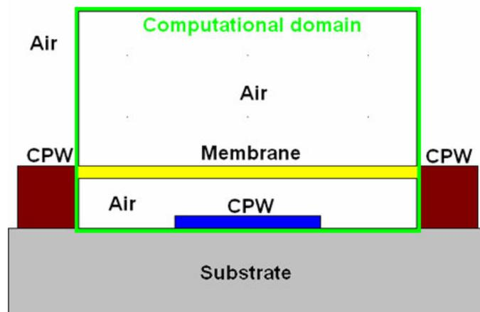
Figure 11.2. The cross-section of the shunt capacitive MEMS switch is presented; The computational domain (green box) is reduced compared to the domain of the mechanical analysis presented in Chapter 8 (more details can be found in text); The abbreviation CPW means the coplanar waveguide (the CPW system consists of two grounded conductors (brown) on the sides and one signal carrying conductor (blue) in the middle [2, 3]).
