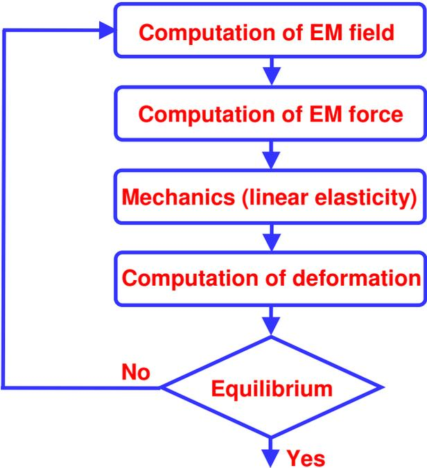
Figure 11.1. The iterative algorithm for the solution of the two-way field coupling between electromagnetics and mechanics is presented; More details can be found in the text.
