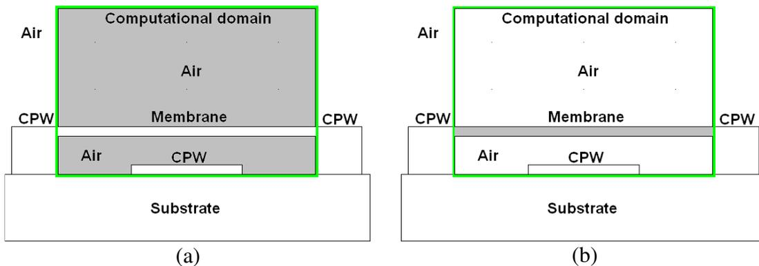
Figure 11.3. The computational domain (gray area) of the electrostatic (a) and mechanical analysis (b); In the electrostatic analysis the membrane is set to the potential zero and the middle conductor of the CPW is set to the input DC voltage ( $V_{IN}$ ); In the mechanical analysis only membrane is under consideration and the touching surfaces between the membrane and the conductors of the CPW are set to be fixed (a mechanical constraint or zero displacement BC).
