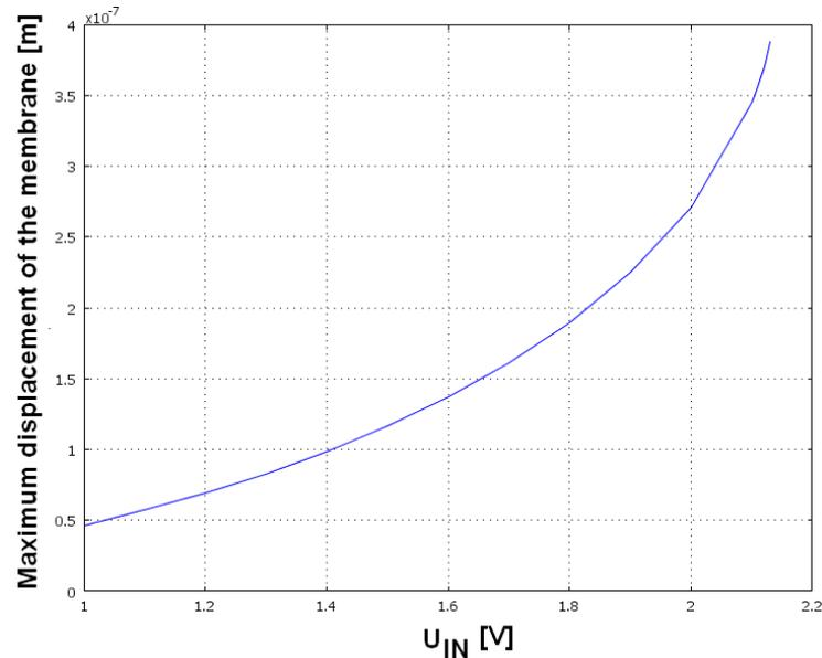
Figure 11.7. The result of the parameter study of the coupled-field problem using the ALE method; The maximum deformation of the membrane with respect to the input DC voltage is presented; The extrapolation of this curve can help us to estimate the pull-in voltage.
