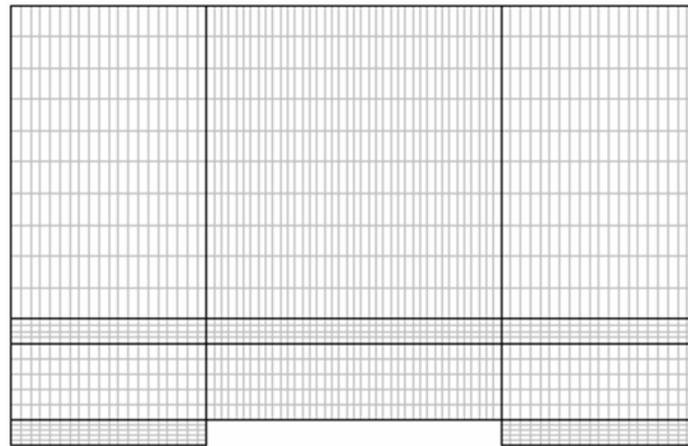
Figure 11.4. The regular mesh covering our computational domain is shown; Such a mesh can partially compensate the negative numerical effect of the large geometric aspect ratio of our structure.
