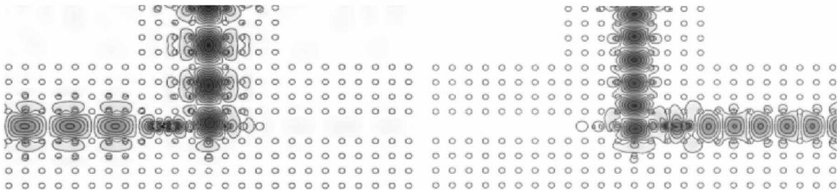
**Figure 3.**  $a = 1\mu m$  ; for right propagation  $a/\lambda = 0.41$  ; for left propagation  $a/\lambda = 0.346$
