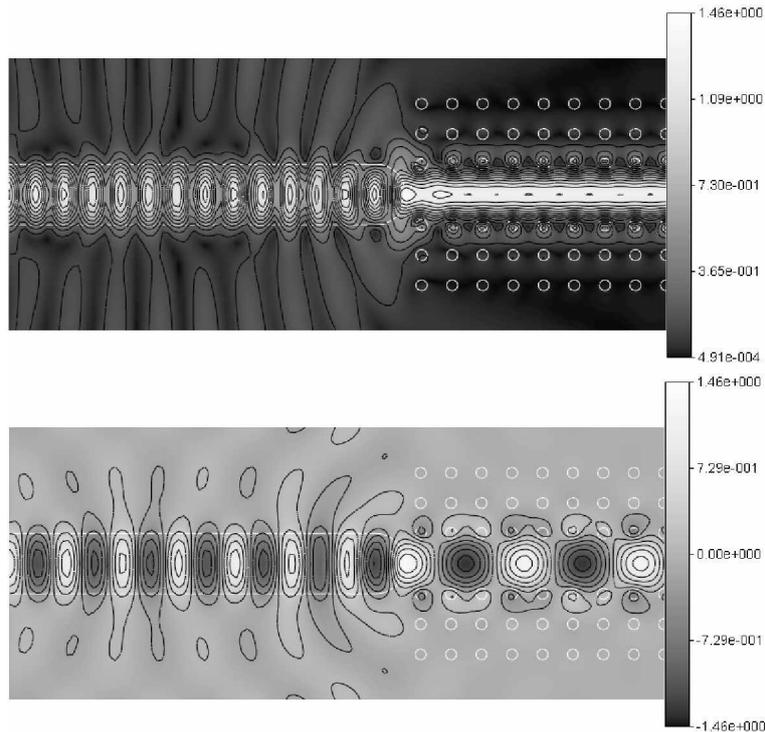
**Figure 4.** Coupling of a slab waveguide into a PhC waveguide at relative frequency  $fa/c=0.38$ ;  $h(\text{diel\_WG})= 3.379$ ;  $h(\text{PC})= 1.644$ ;  $\text{SWR\_WG}(\text{MAS})= 1.718$ ;  $\text{SWR\_WG}(\text{MMP})=1.656$ .
