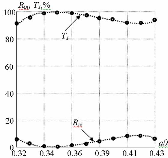
**Figure 2.** Comparison of the MAS (circles) and MMP (dashed lines) model for a 90° W1 defect waveguide bend as a function of the normalized frequency  $a/\lambda$  within the first bandgap. The discrepancy is less than 1% for all frequencies.
