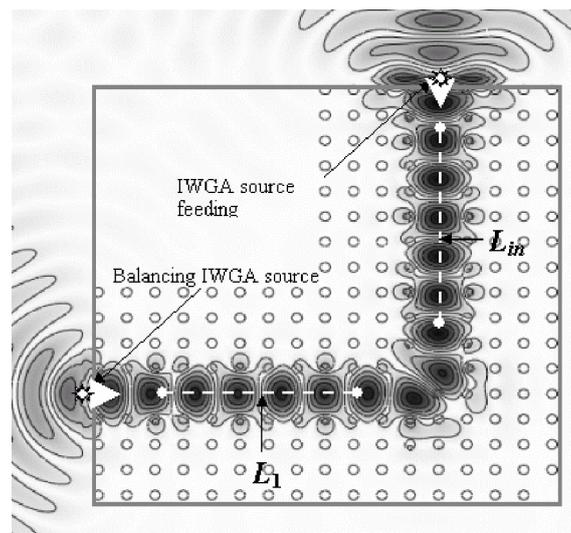
**Figure 1.** MAS simulation of the 90° W1 defect waveguide bend. The gray rectangle outlines the truncation boundary of the finite PhC model. The underlying PhC consists of a square lattice with  $a/\lambda = 0.416$ ,  $\epsilon = 11.56$ , and  $r/a = 0.18$ . (i) MAS simulation; relative error estimate: 0.3%; transmission 91.15%; reflection 8.58%. (ii) MMP simulation; relative error estimate: 0.45%; transmission 91.26%; reflection 8.56%.
