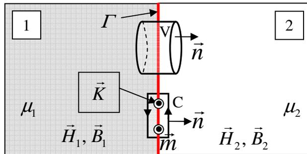
Figure 3.5. Interface between two different materials (materials are different in magnetic sense); V – small cylindrical volume; C – small contour;  $\sigma$  - surface density of electric charge over interface;  $\Gamma$  - surface boundary (interface) between two domains.
