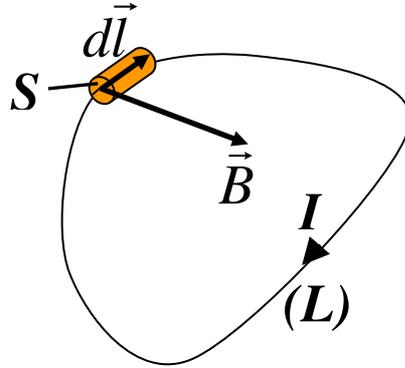
Figure 3.4. A current carrying conductor loop is depicted (L); The conductor loop is exposed to the influence of an external magnetic field with magnetic induction ( $\vec{B}$ ); It is assumed that the conductor has a cross section of constant shape (S) which is much smaller than its length.
