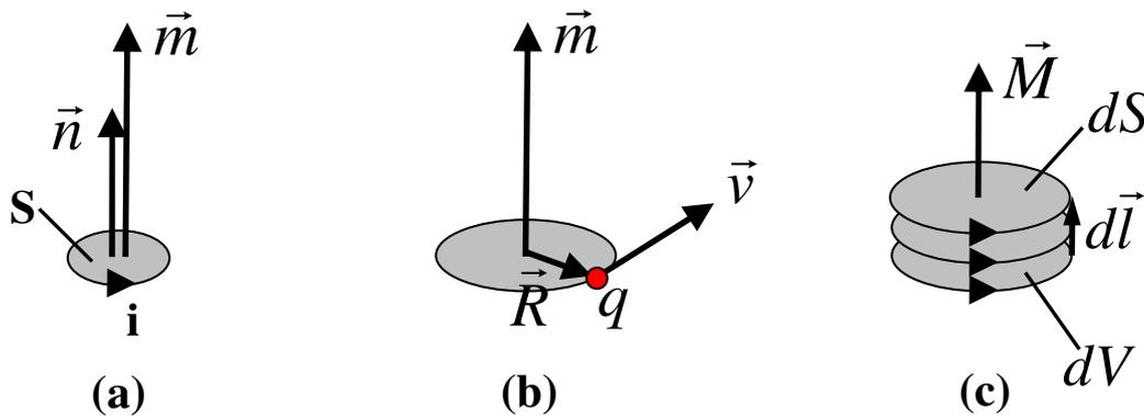
Figure 3.3. The magnetic dipole is depicted; (a) a small current loop as a magnetic dipole; (b) a point charge orbiting around a centre as a magnetic dipole; (c) a macroscopic representation of the magnetic dipoles in a certain material.
