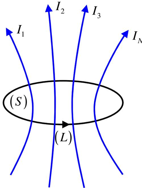
Figure 3.1. Ampère's law;  $L$  - closed integration curve;  $S$  - surface bordered by  $L$  ;
