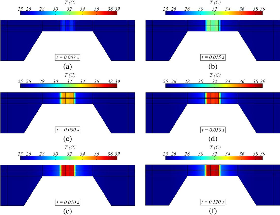
Figure 9.6. Temperature distribution over the structure for different moments in time is shown; The time-moments (a-e) are marked on the time-diagram of heating in Figure 9.5.
