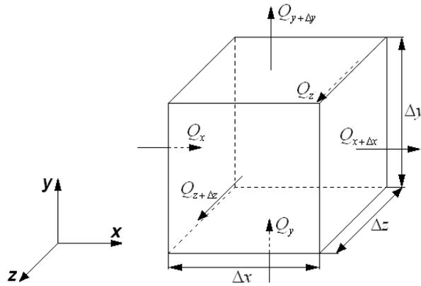
Figure 9.1. An elemental volume in the Cartesian coordinate system used for the derivation of heat transfer equation is depicted.
