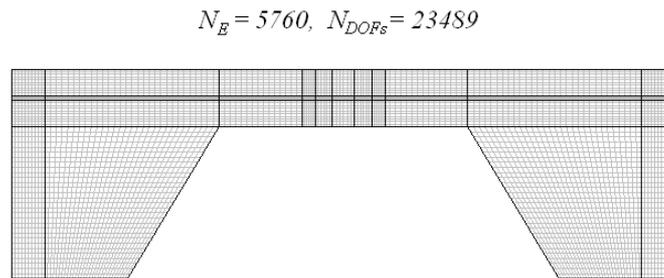
Figure 9.4. A regular rectangular mesh is depicted; The number of degrees of freedom is much larger than the number of elements due to a choice of second order shape functions over the element (8 nodes per rectangular element).
