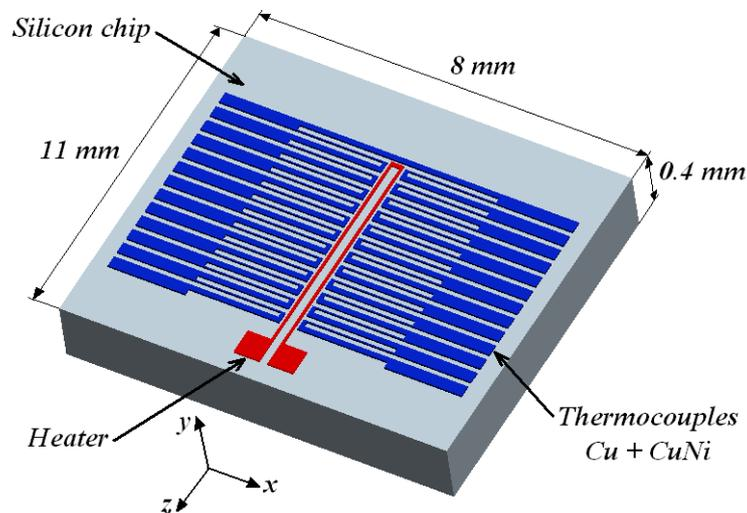
Figure 9.2. A simplified representation of the micro AC/DC thermo-converter described in [3, 4] is shown; The basic constitutive parts of the thermo-converter are the heater (red), the thermocouples (blue) and the silicon wafer (gray); Typical dimensions of the structure are given.
