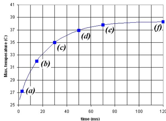
Figure 9.5. The heating diagram of the structure is depicted; The maximum temperature in the structure has been recorded for each time step and visualized (blue line); The characteristic moments of time have been chosen (a-f) and the temperature distributions for each particular case are depicted in Figure 9.6.
