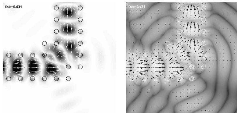
**Figure 5.** 90°-bend based on the single-crystal-layer-waveguide scheme. **Left:** The Poynting vector (linear scale). **Right:** The Poynting vector (logarithmic scale, inverted grayscale). Numerical results:  $R \approx 7\%$  (power reflection),  $T \approx 60\%$  (power transmission),  $A_{rad} \approx 33\%$  (radiation).
