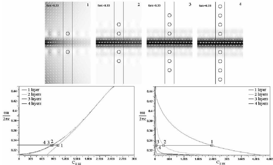
**Figure 4.** Numerical results of complex eigenvalue search for different waveguides. **Top:** Poynting vector field for waveguides with different widths of the PhC walls at relative frequency  $f \cdot a/c = 0.33$ . **Bottom:** Real part (left-hand side) and imaginary part (right-hand side) of the propagation constant.
