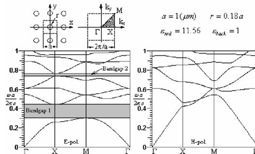
**Figure 1.** Basic properties of a perfect crystal and its band structure; **Top:** Original lattice, 1<sup>st</sup> (irreducible) Brillouin zone, lattice constant and material properties. **Bottom:** Band diagram for E-polarization (left-hand side) and H-polarization. (right-hand side). Bandgaps exist only in the case of E-polarization (gray areas).
