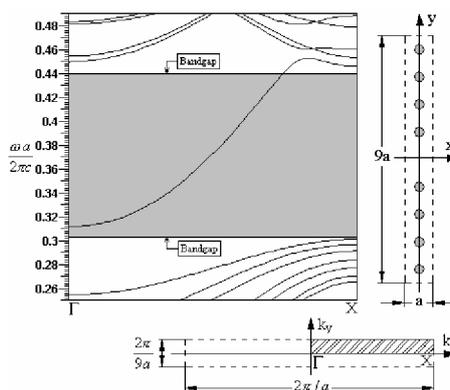
**Figure 2.** Line defect waveguide (vacancies) and detail of the corresponding classical supercell. **Top:** Section of the band diagram around the first bandgap (left-hand side) and supercell (right-hand side). **Bottom:** Detail of the irreducible 1<sup>st</sup> Brillouin zone. Many extended modes appear above and below the bandgap (gray area). They are not interesting for practical applications. A single defect mode (i.e. the defect waveguide mode) covers almost the entire bandgap.
